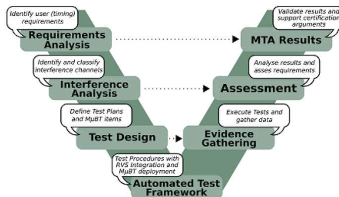
Steps in the V-model software development process applied to multicore timing
